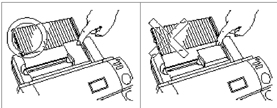
The laminating process is interrupted if the inserted document length is more than 13.8" (350 mm). The color of **Start** button will be changed to orange. Press **Start** to restart the process.
