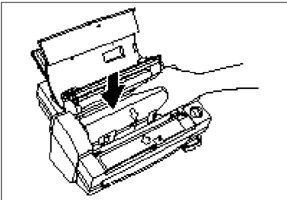
(3) Carefully install the film cartridge, square end down.
