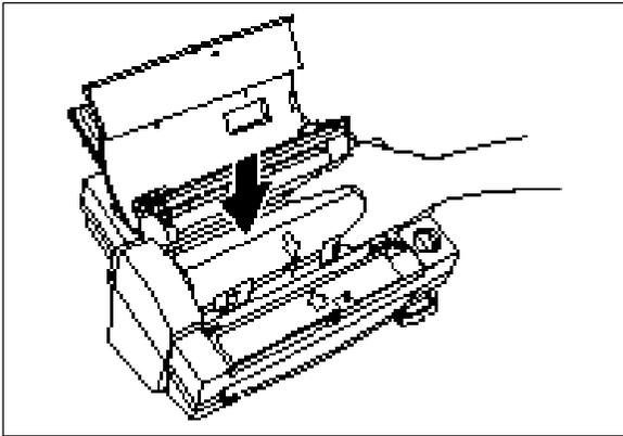
(4) Install the new film cartridge carefully.
