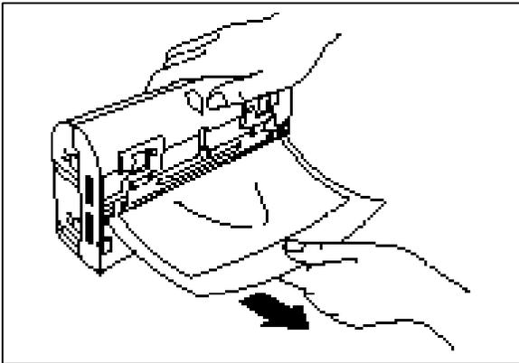
(5) Remove the document from the film slit of the cartridge.
