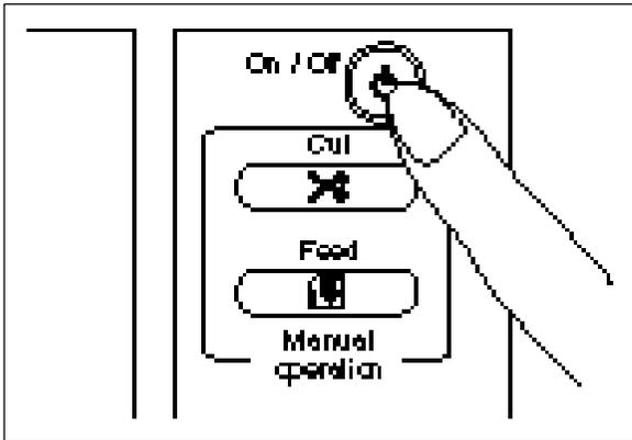
(3) Press the power switch on the control panel to turn it on. The green **Start** button will light up. If the machine does not respond, check the connection of the AC adapter.
