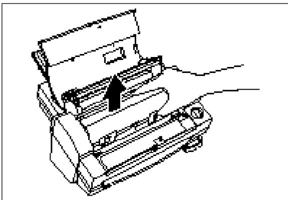
(3) Remove the film cartridge carefully.
