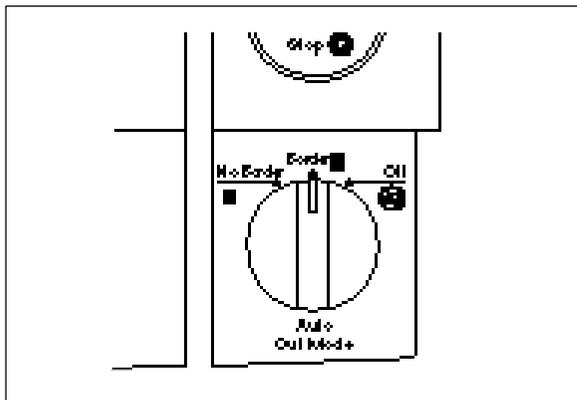
(4) Select the Cut Mode by using Auto Cut Mode selector switch. Please refer to 'How to define the cutting position' page 19.
