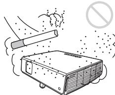
Avoid installing the unit in a very dusty or extremely smoky environment. Otherwise, the air filter will become obstructed, and this may cause a malfunction of the unit or damage it. Dust preventing the air passing through the filter may cause a rise in the internal temperature of the unit. Clean the filter periodically.
