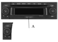
▶ Push the release slide for the control panel (A) to the right.
