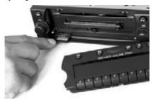
Insert the MMC<sup>TM</sup> into the slot with the printed side up.
