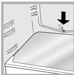
The refrigerator has an automatic defrosting function: water is ducted to the back of the appliance by a special discharge outlet (see diagram) where the heat produced by the compressor causes it to evaporate. It is necessary to clean the discharge hole regularly so that the water
