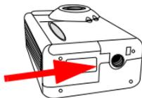
Close battery compartment cover and slide the cover in the direction shown. You will hear a click sound when the cover is firmly closed.
