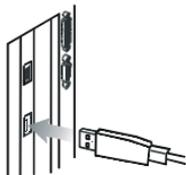
Connect the other end of the USB cable to the USB port on the back panel of your computer and your computer will install DC 1500 to your system as a new drive automatically.
