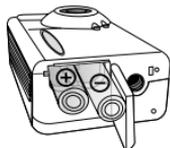
Open the cover and insert two AAA alkaline batteries into the compartment. Note the polarity of the batteries when you install.
