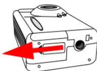
Press the battery cover and then slide the cover in the direction shown.
