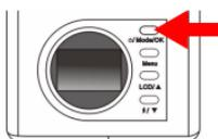
Press the "Power" button for 2 seconds to turn on the power of the camera.
