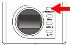
To turn off the power, press the "Power/Mode" button for 2 seconds to turn off the power of the camera. You will see the LCD screen turn blank. Then the power is turned off.
