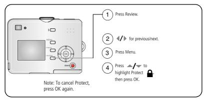
The picture or video is protected and cannot be deleted. The Protect icon  $\mathbf{a}$  appears with the protected picture or video.
