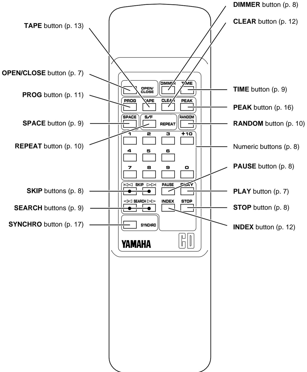
This manual describes how to operate this unit by using the remote control transmitter.
