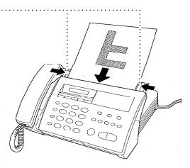
■ The automatic document feeder (ADF) can hold up to 10 pages, feeding each one individually through the fax machine. Use standard (20 lb.) paper when using the ADF; if you're using heavier paper, feed each sheet individually to prevent paper jams.
