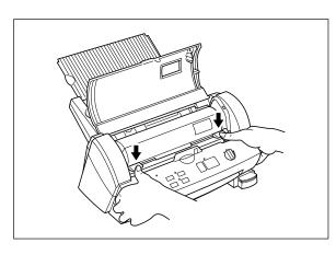
(8) Return the roller holder levers to its original position. Push until it clicks into place.
