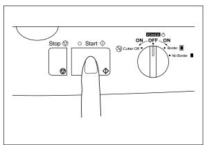
(2) Press Start. The machine will start to laminate your document. When the end of the document is detected the laminating process pauses and the buzzer sounds.
