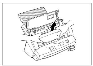
(3) Remove the film cartridge taking care not to grab the cartridge by the shutter.
