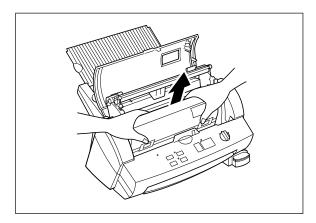
Remove the film cartridge from the machine being careful not to grab the cartridge by the shutter.
