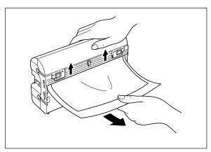
(5) Open the cartridge shutter and remove the document from the film slit of the cartridge.
