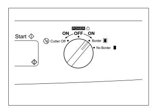
(4) Turn the POWER dial to Cutter Off, Border or No Border to select the cut mode. Please refer to 'How to define the cutting position' page 16.
