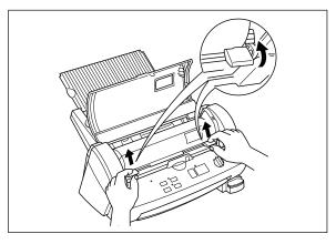
(2) Pull the roller holder levers up and lift the roller holder upwards.
