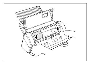
(6) Return the roller holder to its original position and press the roller holder levers as illustrated. You will hear the roller holder click into place.
