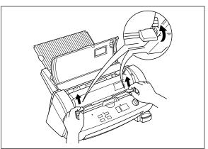
(3) Pull the roller holder levers up and lift the roller holder upwards.
