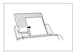
(3) Align the paper with the tab on the right and slide the document guide until it touches the left edge of the document. When laminating an irregularly shaped document, always position the longest edge of the document to the right.
