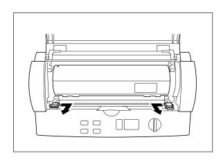
(5) Slide the old side cutter towards the center of the machine. Remove the side cutter.
