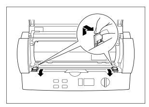
(7) When the cutter is in the correct position lift the tab and bring it upwards towards the front of the machine to lock the side cutter into place.
