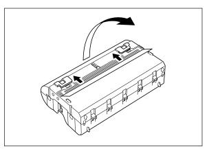
(2) Open the film cartridge by sliding the shutter in the direction of the arrows until it locks into place. Open the film cartridge by gently separating the clear top cover from the gray bottom cover.
