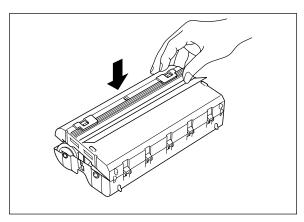
(6) Close the film cartridge. Making sure that the leading edge of the film sticks out of the film slit.
