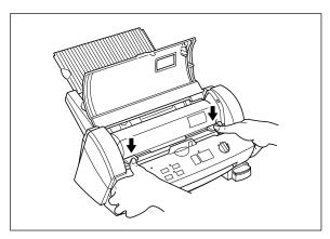
(10) Return the roller holder to its original position and press the roller holder levers as illustrated. You will hear the roller holder click into place.
