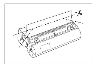
(6) Remove any excess laminating film by cutting along the engraved "cutting line" on the cartridge before reinserting the cartridge.
