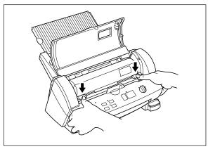
(5) Return the roller holder to its original position and press the roller holder levers as illustrated until it is secured into position. You will hear the roller holder click into place.
