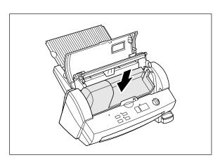
(4) Place the cartridge adapter into the machine as illustrated.
