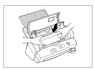
(9) Install the cartridge into the machine.
