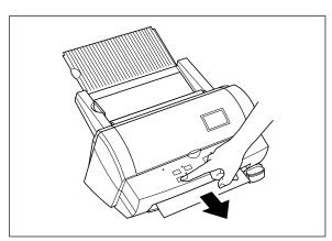
(2) Press the Feed button to feed the document manually. The Feed button is a self-repeating key. The document will continue to be fed until the Feed button is released. Keep pressing the Feed button until you see the end of the document.
