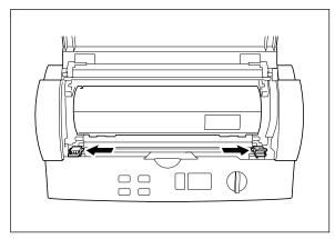
(6) Place the new side cutter on the metal bar and slide it towards the side of the machine.
