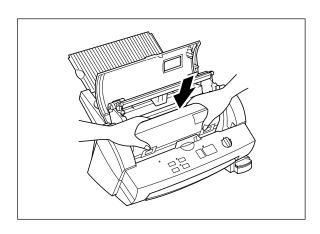
(4) Carefully install the new film cartridge, square end down, film slit facing towards the front of the machine.
