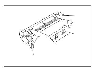
(7) Press on the two shutter buttons marked "PUSH" to release the shutter.
