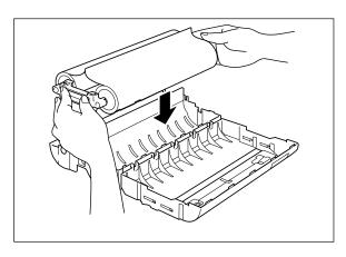
(4) Take the new refill roll of film from the sealed package. Remove the separator sheet. Holding the yellow colored plastic side holders of the film roll. Place the film into the cartridge as illustrated. The film can only be placed into the cartridge in the correct direction.
