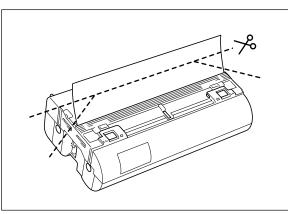
(8) The top edge of film should be aligned with the cutting line of the cartridge. If any film extends beyond the cutting line, cut away the excess film as illustrated before installing the cartridge into the machine.
