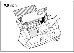
(5) Place the 9.0 inch or 4.8 inch cartridge into the machine.
