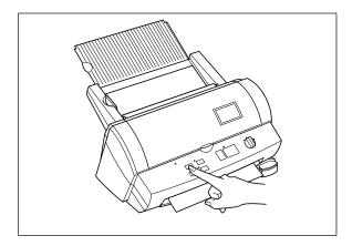
(3) Press the **Cut** button. The document will be cut at its current position.
