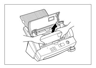
(3) Remove the film cartridge carefully.
