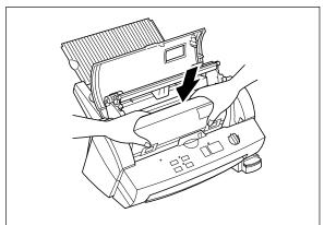
(7) Place the film cartridge into the machine.
