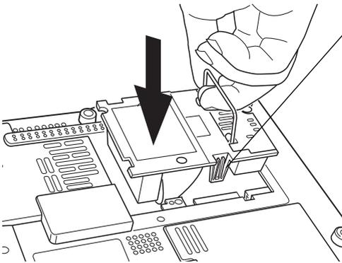
Make sure that the grooves on either side of the lamp cartridge align properly with the grooves on either side of the lamp housing.
