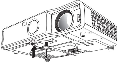
2. While holding down the release button, raise and lower the front of the projector until the elevation adjustment foot is approximately the length you need.
