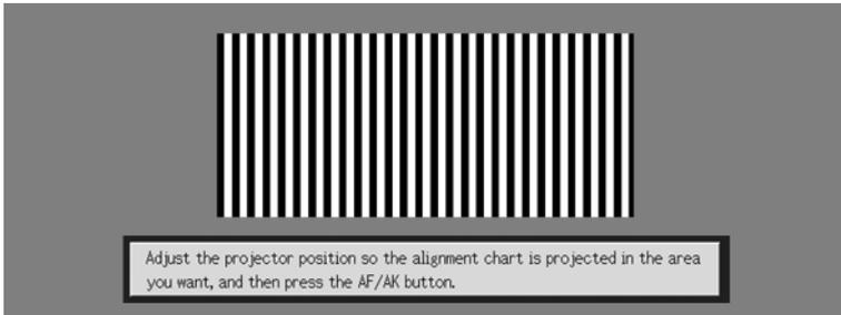
2. Adjust the angle and position of the projector as required so the projected chart fits within the screen area.
