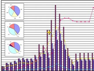
2. Use the remote controller's cursor keys to move the cross cursor to the part of the image that you want in the center of the enlarged image.
