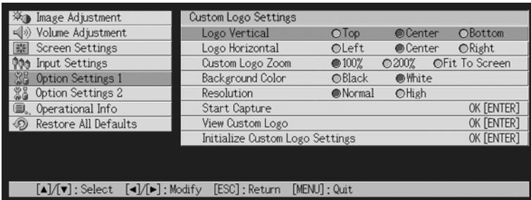
4. Use the [▲] and [▼] keys to select “Start Capture”, and then press the [ENTER] key.
