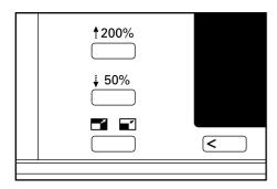
Press the cursor up or down key to select the desired magnification ratio and then press the enter key.
