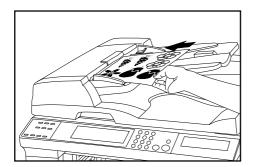
Set the original with the side to be copied facing downward. Be sure to align the original with the original size scales.
