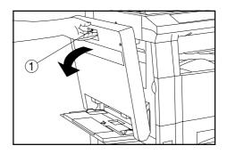
Hold the switchback guide handle ② and open the switchback guide, and then remove the misfed paper.
