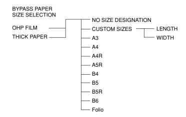
Press the cursor right or cursor left key and select the paper length, which is shown highlighted. The paper length can be set to any value from 100 to 297 mm in 1 mm increments.
