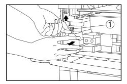
Close the opening of the waste toner tank with its seal.
