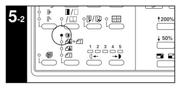
To have the copy exposure adjusted automatically, press the copy quality selection key and set the auto exposure mode. The Auto Exp. indicator will light. In the auto exposure mode, the brightness of the original is detected and the most suitable exposure selected. It is also possible to make clean copies without the original background or color.
