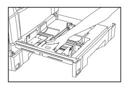
Hold the width adjustment lever and move it to align the width guide with the required paper width.
