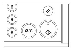
Replace the original and press the Start key. Scanning of the originals will start. Carry out the same procedures to the originals of which copying will be performed, and finally, press the enter key. Copying will start.
