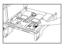
Hold both sides of the length adjustment plate and move it to align with the required paper length.
