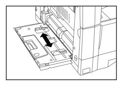
Open the envelope and set it with the print side face-down and its flap opposite to the insertion slot and then insert it along the insert guide as far as it will go.
