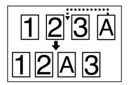
When copying ends, press the Interrupt key again, and replace the newly copied original(s) with the one(s) removed before. Then, press the Start key.
