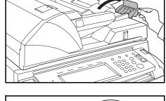
Ensure that loaded originals do not exceed the level indicated. Exceeding the maximum level may cause the originals to jam.
