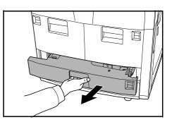
Using the paper length adjusting tab, move the plate to 2 fit the paper.
