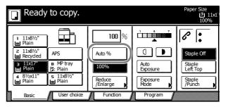
3 Press the **Start** key. The image will be automatically reduced or enlarged for copying onto the selected paper.
