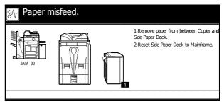
**1** Press the top button of the side feeder and detach the side feeder from the copier.
