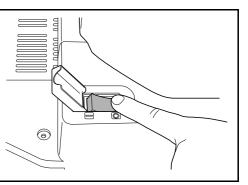
When turning off the main power switch, press the **Power** key on the operation panel to off (O). Make sure that the **Power** lamp is off before turning off the main power switch. Turning off the main power switch before pressing the **Power** key to off may cause damage to the equipped hard disk.
