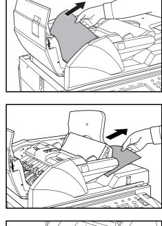
If it is difficult to remove the original, turn the feed dial. The original will be pushed to a place where it is easier to remove.
