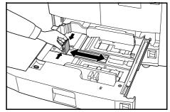
**3** Holding the paper width adjusting tab both ends, move the paper width guide to fit the paper.
