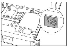
**5** Insert the appropriate paper size card in the slot to indicate the size of the paper inside.
