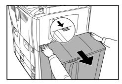
2 Remove the paper jammed in the connecting slot of the side feeder.
