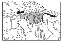
**3** Let go of the toner container release lever and pull the used toner container until it can be removed.
