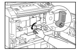
4 Turn the knob A3 counter-clockwise at least 8 times. Jammed paper will be pushed to the paper conveyor.
