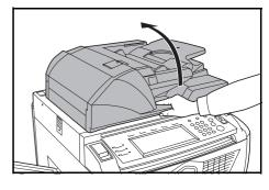
2 Place the original. Put the copying side facedown and align it flush against the original size indicator plates with the back left corner as the reference point.
