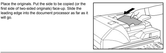
IMPORTANT: Confirm that the original width guides exactly fits the originals. If there is a gap, readjust the original width guides. The gap may cause the originals to jam.
