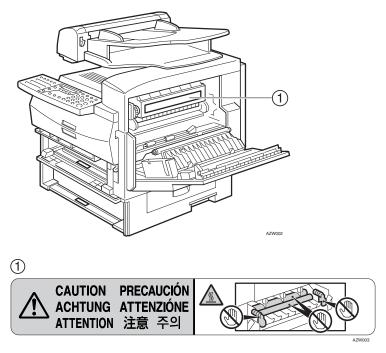
High temperature. Be careful of hot parts when clearing paper jams.
