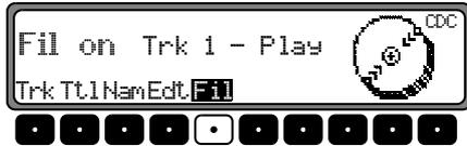
For the Silverstone 2660 CD changer, the individual tracks of the current CD can be selected using the right rotary control **◀**. By pressing the right rotary control **▶** selection can be made between **Play** (Title unfiltered) and **Skif** (Title filtered out).
