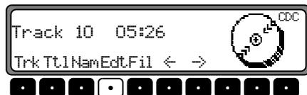
The individual entries can be selected by pressing the multifunction buttons **<-** and **->**, selecting the desired position (inverse editing symbol).
