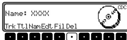
By pushing the multifunction button **Del**, the name can now be deleted.
