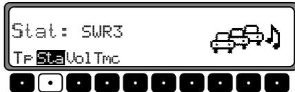
Using the right rotary control, select the desired TP station and press to confirm. After a short delay and without actuation, the selected station is accepted.
