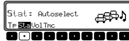
Select **Autoselect** with the right rotary control and press to confirm. After a short delay and without actuation, the direct programming is deleted.
