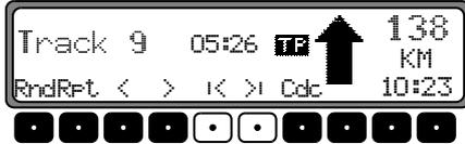
By pressing the multifunction button repeatedly, several tracks can be skipped over in forward or reverse directions. Once the last track has been reached in the forward direction, the unit switches back to the first track. Analogously, it switches from the first track to the last track when going backward.
