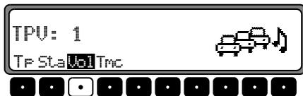
With the right rotary control
