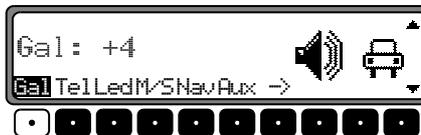
With the GAL setting, the start of volume adjustment can be specified according to vehicle speed.
