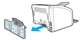
4 Insert the new separation pad, and screw it in place.
