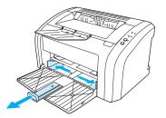
**3** Place the envelopes with the side to be printed facing up and the top edge along the left media guide. Stack up to 15 envelopes.
