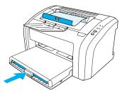
**3** After side one has printed, remove the remaining paper from the input tray, and set it aside until after you finish your manual duplexing job.
