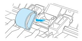
6 Position the new or cleaned part in the slot of the previous pickup roller. See <u>Cleaning the</u> <u>pickup roller</u> for instructions.Circular and rectangular pegs on each side prevent you from incorrectly positioning the pickup roller.
