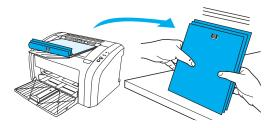
5 Place the stack back in the input tray. Side one should be facing down with the bottom edge feeding into the printer first. Replace the priority input tray.
