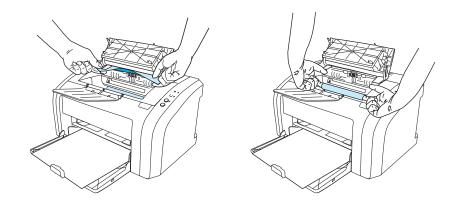
4 When you have removed the jammed media, replace the print cartridge, and close the print cartridge door.
