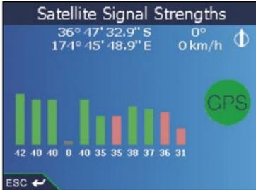
The circle on the right side of the screen displays green when there is a valid fix (2D or 3D), and red when no fix is available. A fix will be obtained more quickly if the vehicle is stationary than if it is moving.
