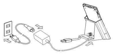
**Method 2.** Connect the supplied AC adapter and the Toshiba Pocket PC as shown in the figure below.
