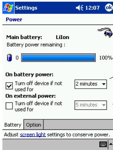
Options are 1, 2,3,4, and 5 minutes until device will turn off in battery-powered mode if not used. Check box to left to engage this feature.
