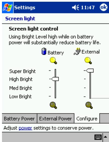
Tap and set the front light brightness level by move the cursor up or down. If Power Save is activated, the front light turns off.
