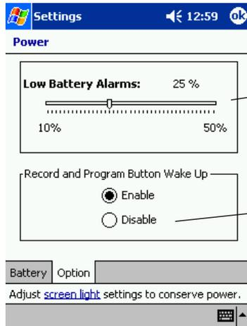
Battery alarm can be adjusted to go off from 10% to 50% of full charge.
