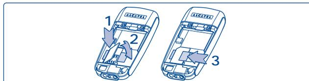
Before inserting the SIM card into the slot, push the SIM card catch to release it as shown (1-2). Lift the catch and place the SIM card into the slot with care.
