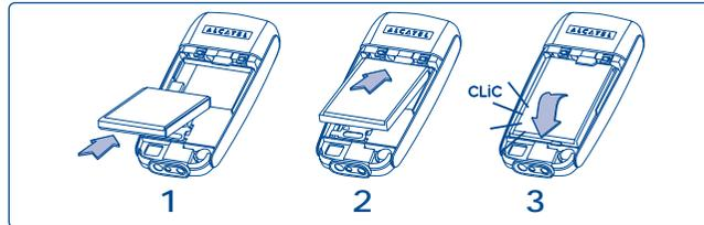
Align the tab on top of the battery with the slot in the battery compartment of your phone. Press down the battery until the latch is completely locked.
