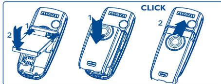
Insert and engage the battery, then close the telephone cover.
