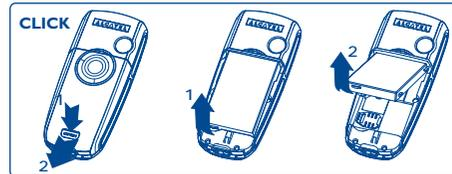
Unclip the cover, then the battery and remove it.
