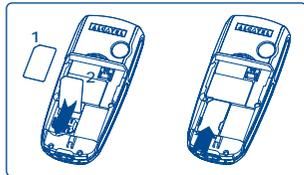
Place the SIM card with the chip facing downwards and slide it into its housing. Make sure that it is correctly inserted.
