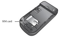
A SIM card can be easily damaged if its metal contacts become scratched. Therefore, take special care when holding or inserting it.
