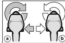
The rotational direction switch **8** is used to reverse the rotational direction of the machine. However, this is not possible with the On/Off switch **9** actuated.
