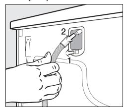
■ Unclip the drain hose, 1, and pull it off the holder 2
