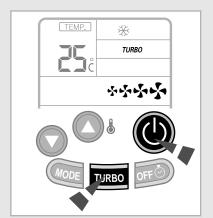
The Turbo cooling/heating function is used to cool or heat your room as quickly as possible.
