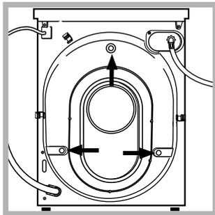
3. Remove the three protective screws and the rubber washer with the respective spacer, situated on the rear of the appliance (see figure).
