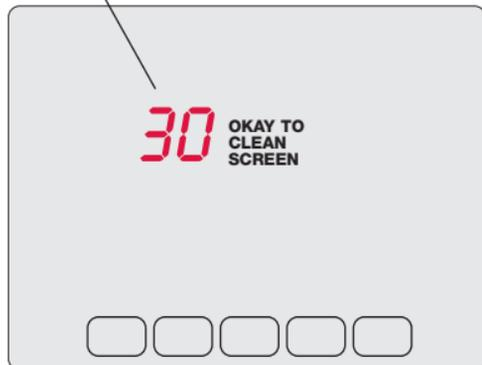
Press **SCREEN** to lock the screen for cleaning. The screen will remain locked for 30 seconds so you can clean the screen without changing any settings.
