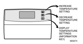
2. To raise the temperature setting, press the A key. When in the cooling mode, raising the temperature before you leave for work or school also lowers. your energy costs.
