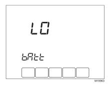
NOTE: Although the thermostat has a low battery indicator, replace the batteries once each year to prevent leakage and to prevent the thermostat and heating/cooling system from shutting down due to lack of battery power in the thermostat.
