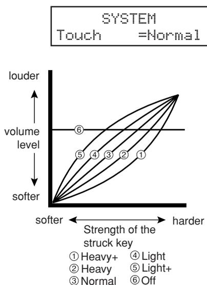
This parameter adjusts the touch response curve of the keyboard.
