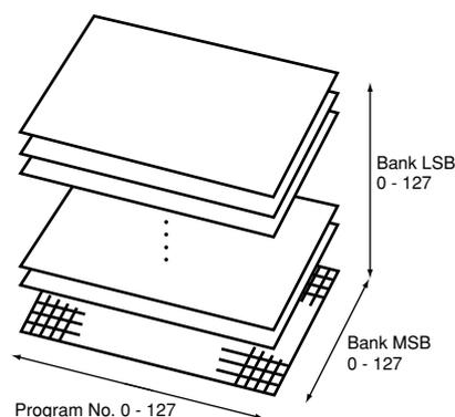
This is a 3D image of the expanded program change system with the MSB and LSB. To use these efficiently and correctly, refer to the operation manual of any external MIDI sound modules that are connected to the MP4.
