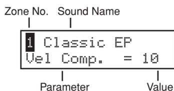
Zone parameters can be edited individually for each zone. There are two parameter groups, Internal parameter group and External parameter group. If a zone is set to Int, only Internal parameters are available for editing. If a zone is set to Ext, only External parameters are available for editing. If a zone is set to Both, both Internal and External parameters are available for editing.
