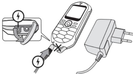
1. Once the battery and battery cover are clipped on the phone, plug the connector of the charger
