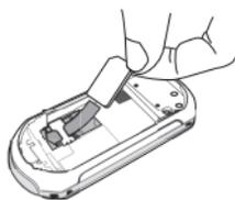
3. Slide the battery into its slot, metallic connectors downwards, until it stops. Then lock it by pushing it downwards.
