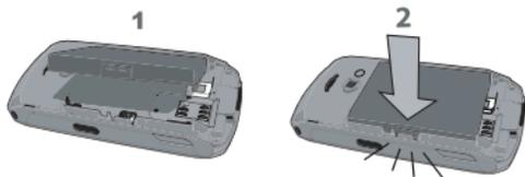
Replace the back cover as shown below: hook the housing into the hinge on the top of the phone, then press the bottom down until the latch catches.
