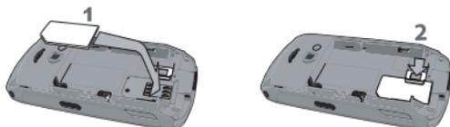
Replace the battery as shown below, connectors downwards.
