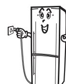
3. Keep it ready and after 1 hour, plug in the power supply. Please refer to the upper indication and conduct relative operations.
