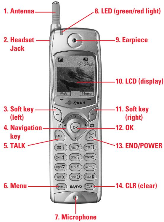
1. **Antenna:** The voice on the other end sounds clearest when the antenna is all the way up.
