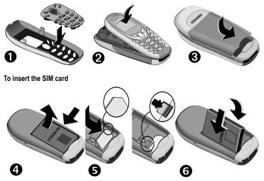
Insert SIM card in the opening, contacts pointing downwards (make sure the angled corner is in correct position **⑤**). Push gently until it engages **⑥**.
