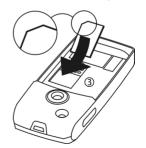
Insert the battery sideways into the phone <sup>(4)</sup>, then press it downwards <sup>(5)</sup> until it clicks into position.
