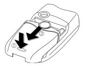
Place the SIM card in front of the slot with the contact surface facing downwards. Then press the SIM card slightly to push it in ③ (ensure that the chamfered corner is in the correct position).
