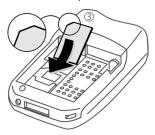
Insert the battery into the phone 4, then press it downwards 5 until it engages.
