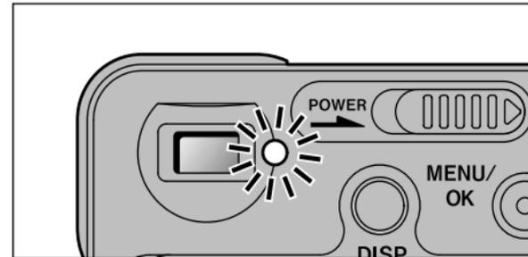
When the viewfinder lamp is lit orange or blinking green, data access (downloading) is in progress. Never open the slot cover or disconnect the cable during data access. This can prevent data downloading and cause camera malfunctions.
