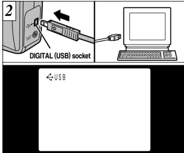
Fit the small plug on the special connection cable into the DIGITAL (USB) socket on the camera and then plug the other end of the cable into the USB socket on your personal computer. When you switch the PC on, “USB” appears in the upper left corner of the LCD monitor.
