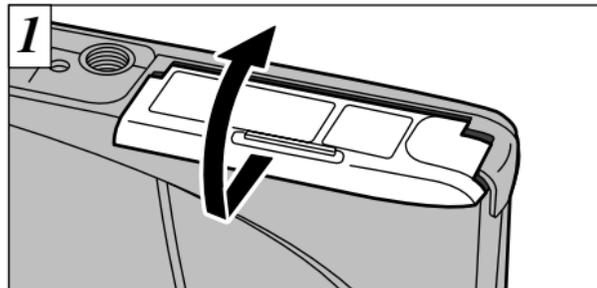
Slide the battery cover in the direction of the arrow and open the cover.
