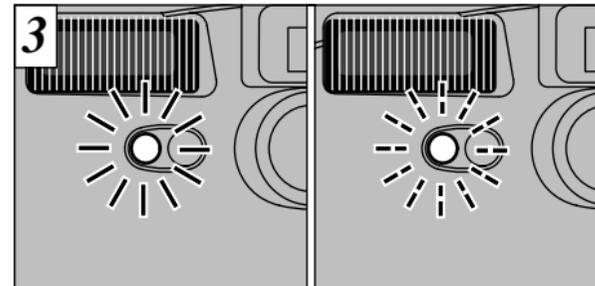
**3** The self-timer lamp lights for 5 seconds, blinks for 5 seconds, then takes the picture.
