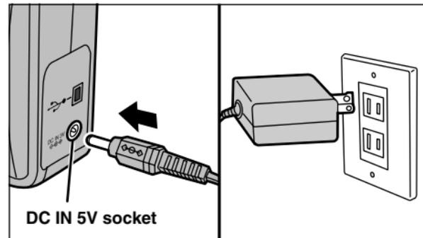
To shoot or play back images without depleting the battery charge, use the special AC Power Adapter AC-5V/AC-5VH. Check that the camera is switched off and then plug the AC power adapter connector into the "DC IN 5V socket" on the camera. Then plug the AC power adapter into the power outlet.
