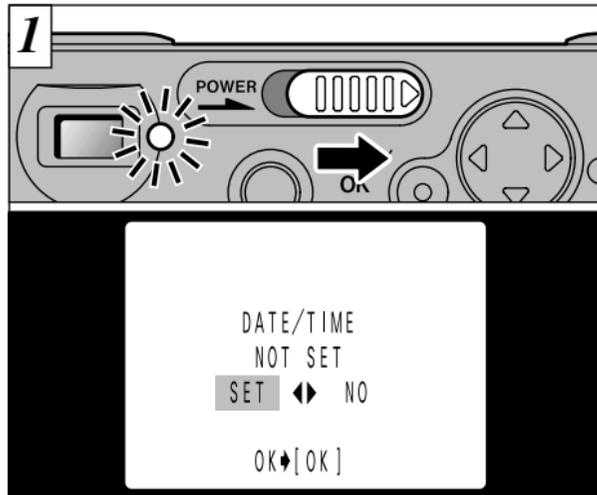
Slide the POWER switch in the direction of the arrow to switch the camera on or off. The viewfinder lamp lights [green] when you switch the camera on.
