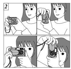
Loop the strap over your wrist, brace your elbows against your body and grip the camera firmly in both hands. When you are holding the camera on its side, hold it so that the shutter button is at the top.
