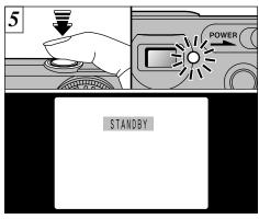
If the green viewfinder lamp stops blinking and stays lit or "[TANDBY]" appears on the LCD monitor when you press the shutter button down halfway, the exposure setting (AE lock) is completed ( $\Rightarrow$ P.22).
