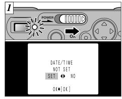
Slide the "POWER" switch in the direction of the arrow to switch the camera on or off. The viewfinder lamp lights [green] when you switch the camera on. If you have not set the date, a confirmation screen appears. Press "◀" or "▶" to select the desired option and then press the "MENU/OK" button.
