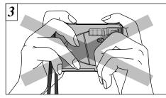
Ensure that your fingers or the camera strap do not obscure the lens, flash, or flash control sensor.
