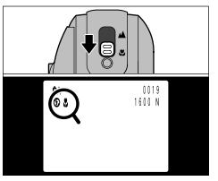
When you set the Normal/Macro selector button to the "" icon, "" appears on the LCD monitor and the camera switches to Macro photography.
