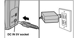
To shoot or play back images without depleting the battery charge, use the special AC Power Adapter AC-5VH/AC-5V.
