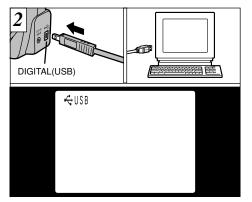
Insert the small plug on the end of the special USB cable into the digital (USB) socket on the camera and then plug the other end of the cable into the USB socket on your PC.
