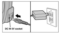
If there is a power socket handy, use the special AC Power Adapter AC-5V/AC-5VH (sold separately) so there is no need to worry about the batteries running out during playback (\$\infty\$P.13, 66).
