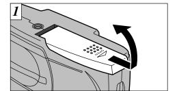
Slide the battery cover in the direction of the arrow and open the cover.
