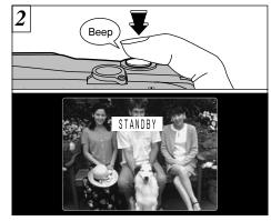
Position the AF frame over the subject and press the shutter button. The camera focuses on the subject in the frame and self-timer starts to run.
