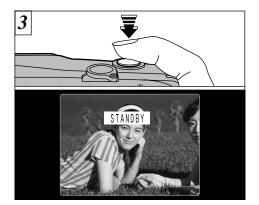
Press the shutter button down half way (AF/AE lock) and check that "STANDBY]" is displayed on the LCD monitor (or that the green viewfinder lamp stops flashing and remains lit).
