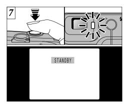
Press the shutter button down halfway. Image focusing is complete when "STANDBY" appears on the LCD monitor or the viewfinder lamp glows green.
