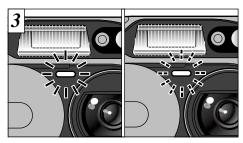
The self-timer lamp lights for 5 seconds, blinks for 5 seconds, then takes the picture.
