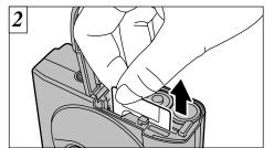
Taking care that the batteries do not fall out of the camera, grasp the SmartMedia and pull it out.
