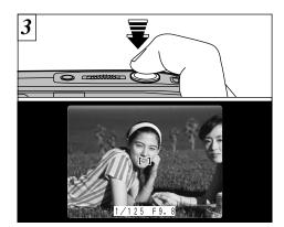
Keep the shutter button held down half way (AF and AE locked) and check that the AF frame is smaller and that the shutter speed and aperture settings are displayed (and that the green viewfinder lamp has stopped blinking and remains lit).
