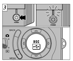
When you press the "o" (power) button on the cradle, the camera is connected to your PC as a removable disk drive and the power lamp on the cradle lights. "DSC" also appears on the display panel.
