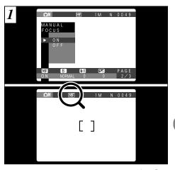
This function can be selected in the "C . AM" and "Qu" photography modes. When the camera cannot focus in AF mode, use this mode to set the focus and take the picture.
