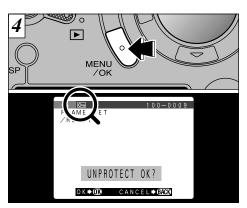
Press the "MENU/OK" button to protect the file. The "Om" icon appears on the LCD monitor. To remove the protection, press the "MENU/OK" button again.
