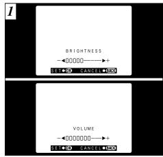
When you use the "LCD BRIGHTNESS" or "VOLUME" settings, an "adjustment bar" appears on the LCD monitor.
