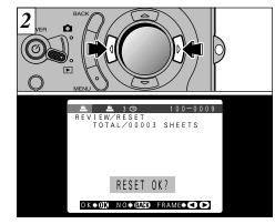
Pressing "◀" or "▶" plays back only the frames 4 for which the number of prints has been specified, allowing you to check the settings for each frame.
