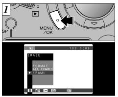
Press the "MENU/OK" button to display the menu on the LCD monitor.
