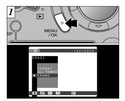
Press the "MENU/OK" button to display the menu on the monitor.
