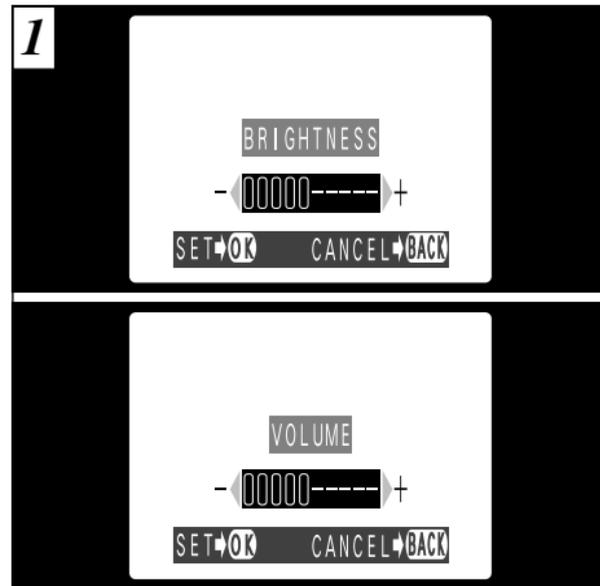
When you use the “LCD BRIGHTNESS” or “VOLUME” settings, an “adjustment bar” appears on the LCD monitor.
