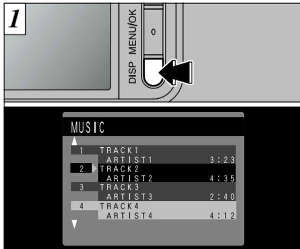
Press the “DISP” button on the camera during music playback to display a list of the tracks on the LCD monitor.
