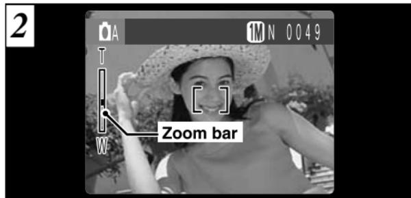
A “zoom bar” appears on the screen. If the image goes out of focus during zooming, press the shutter button down halfway to make it easier to check the shot.
