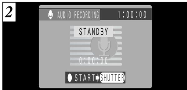
The available audio recording time is shown in the top-right corner of the LCD monitor, while the elapsed recording time and the “STANDBY” message are shown in the center of the LCD monitor.
