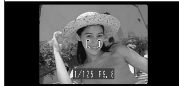
When you press the shutter button down halfway, focusing is complete when the AF frame on the LCD monitor becomes smaller, the shutter speed and aperture setting appear, and the green viewfinder lamp stops blinking and remains lit (→P.28).
