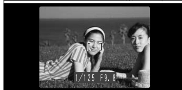
Keep holding the shutter button down halfway (AF/AE lock). Check that the AF frame on the LCD monitor shrinks and that the shutter speed and aperture setting are displayed (the viewfinder lamp (green) changes from blinking to steady).
