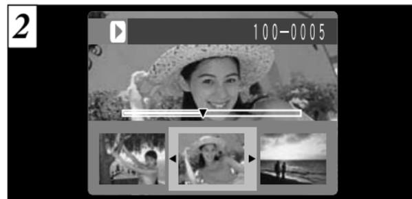
During fast forward, 3 frames are shown together in miniature on the LCD monitor. When you stop fast forward, the image inside the orange frame is displayed on the LCD monitor in normal playback mode.
