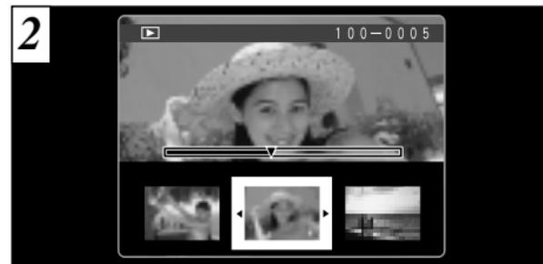
2 During fast forward, 3 frames are shown together in miniature on the monitor. When you stop fast forward, the image enclosed in the cursor (the orange box) is displayed on the monitor as a single image.
