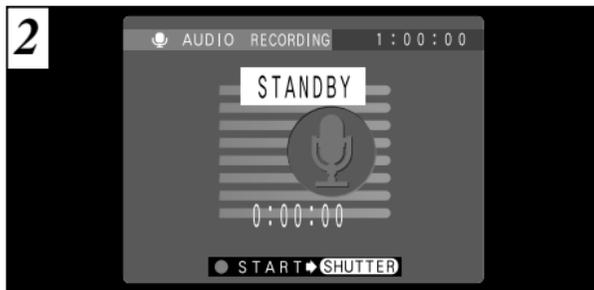
The available audio recording time is shown in the top-right corner of the LCD monitor, while the elapsed recording time and the “STANDBY” message are shown in the center of the LCD monitor.
