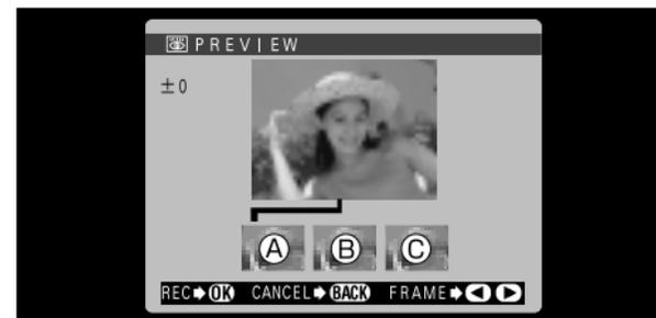
A preview screen appears when you take a picture. **A** is correctly exposed, **B** is overexposed and **C** is underexposed. To record the images, press the “MENU/OK” button. To proceed without recording the images, press the “BACK” button. You can also select the image to be recorded. See P.97 for details.
