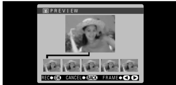
A “PREVIEW” screen is always shown when you take pictures in this mode. The images are arranged from left to right in the order they were taken. To record the images, press the “MENU/OK” button. Do not to record the images, press the “BACK” button. You can also select the image to be recorded. See P.97 for details.
