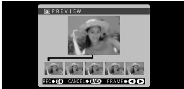
A “PREVIEW” screen is always shown when you take pictures in this mode. The images are arranged from left to right in the order they were taken. To record the images, press the “MENU/OK” button. Do not to record the images, press the “BACK” button. You can also select the image to be recorded. See P.97 for details.
