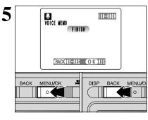
After 30 seconds of recording, " $\fbox{FINISH}$  appears on the LCD monitor.
