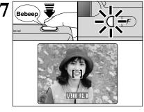
Pressing the Shutter button down halfway, the camera emits a short double-beep and focuses on your subject. At that point, the AF frame on the LCD monitor becomes smaller and the camera sets the shutter speed and aperture (the viewfinder lamp (creen) stops blinking and remains lit).
