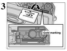
Align the gold marking on the xD-Picture Card slot with the gold contact area on the xD-Picture Card and then push the card firmly all the way into the slot.
