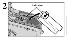
Load the Rechargeable Battery NH-20 correctly as indicated by the polarity icons.
