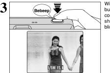
Without moving the camera, press the Shutter button down halfway (AF/AE lock). Focusing is complete when the AF frame on the LCD monitor shrinks and the viewfinder lamp (green) stops blinking and remains lit.
