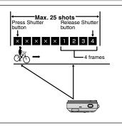
This mode allows you to release the shutter up to 25 times (at intervals as short as 0.3 seconds) and record the last 4 frames.
