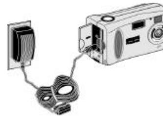
**Note:** If you want to use battery power, disconnect the AC power adapter from the power source and the camera. If the AC power adapter is connected to the camera, even if it is not connected to a power source, the camera cannot draw battery power.
