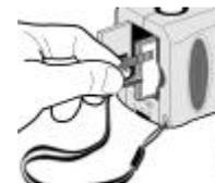
1. Attach the clip on the wrist strap to the memory card. Check that the clip is gripping the card.
