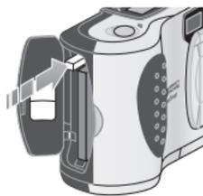
4. Insert the new memory card so that the front of the card faces the front of the camera and the edge with pinholes is placed into the camera first.
