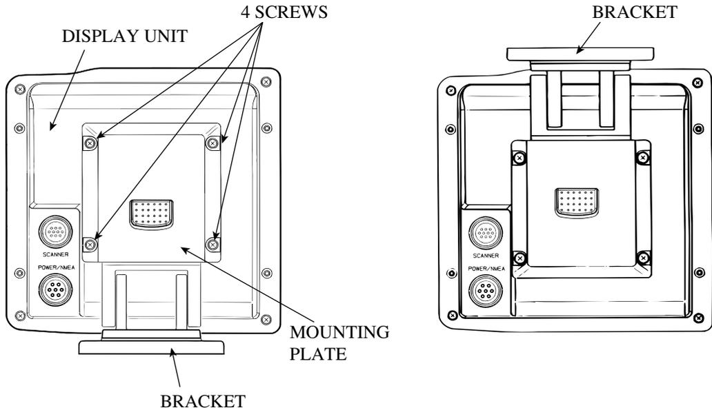
The display unit is separated from the bracket in the shipping carton. Install the display unit by sliding it onto the bracket until it is fully seated.
