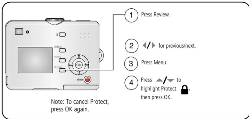
The picture or video is protected and cannot be deleted. The Protect icon
